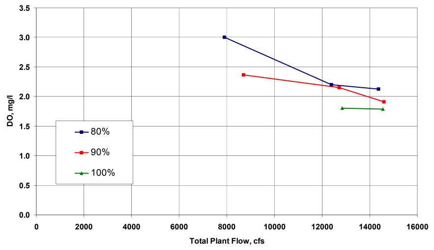
Before hub baffles were added, the minimum DO was 0.4 mg/L.
