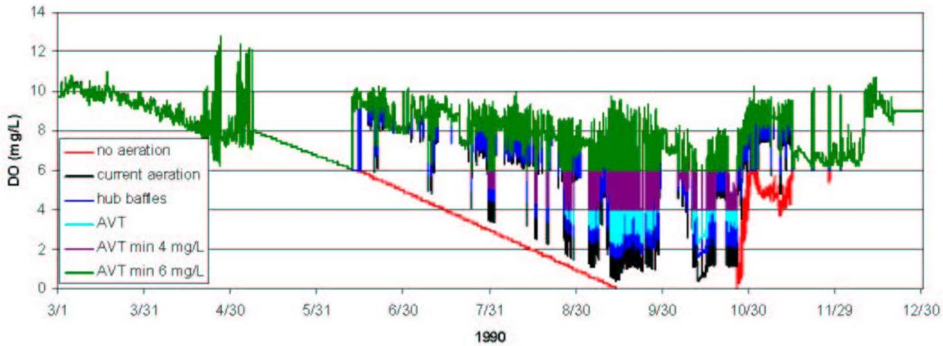
Figure 10: Modeled Release DO and Fish Growth for Aeration Scenario – Wet Year (1990)
