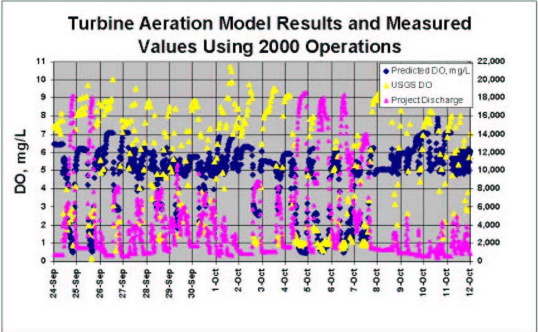
**Figure 4: Turbine Aeration Model Predictions for Discharges from Saluda Hydro Compared to Data from the USGS Monitor 1,000 Feet Downstream from the Dam**
