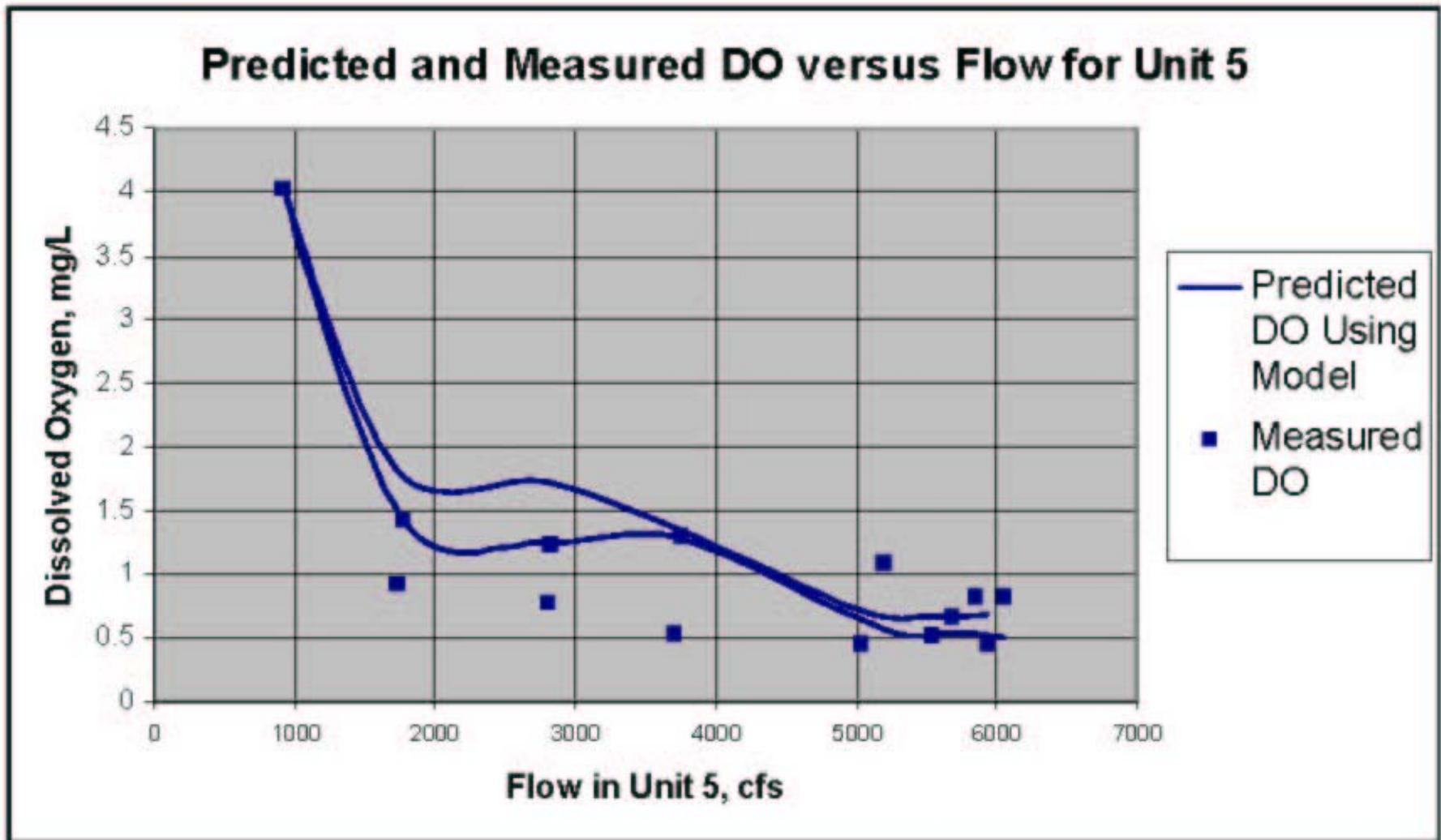
Figure 3: Model Predictions Compared to Data Collected on DO at Various Unit Flows for Unit 5
