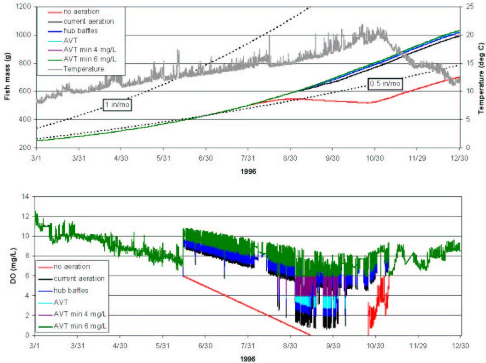
Figure 11: Modeled Release DO and Fish Growth for Aeration Scenario – Moderately Wet Year (1996)
