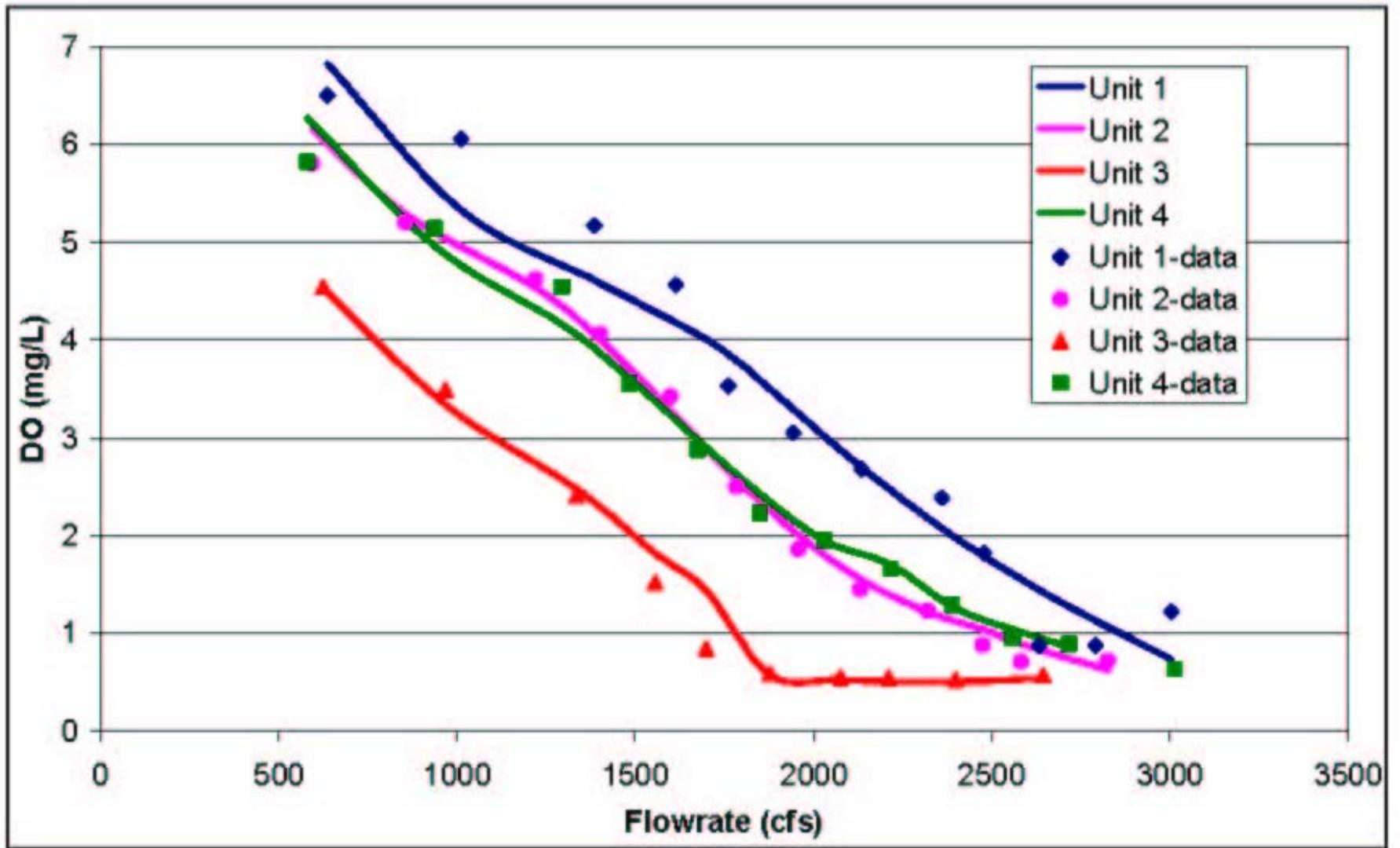
Figure 2: Model Predictions Compared to Data Collected on DO at Various Unit Flows for Units 1-4
