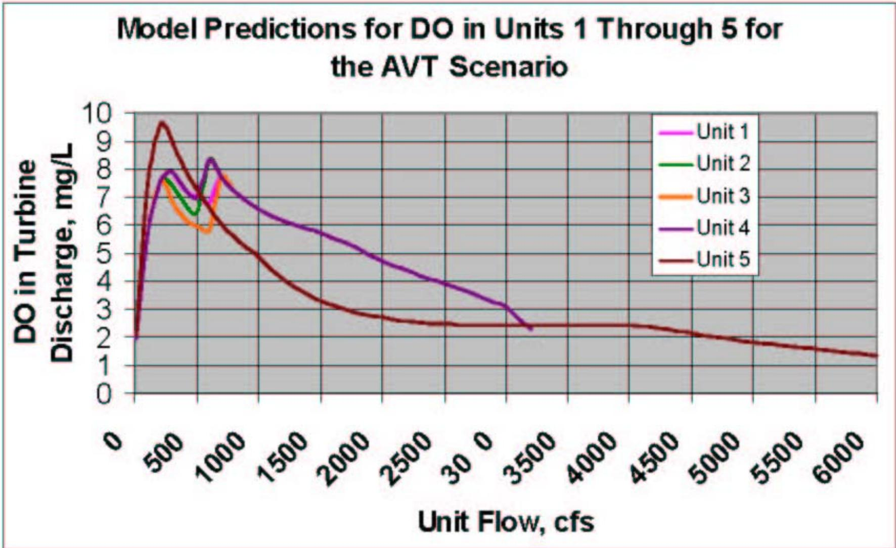
Figure 6: Predicted DO at Various Flow Levels for Each Unit Assuming New Aerating Turbine Wheels Have Been Installed on Units 1-5
