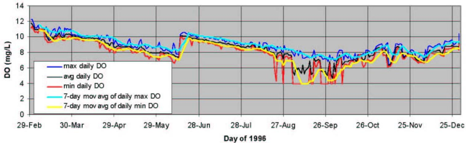
**Figure 7: Summary of DO Metrics from a Model Run for the Year 1996 Assuming that New Aerating Turbines were Installed and Some Supplemental Aeration System was Used to Maintain a Minimum DO of 4 mg/L**
