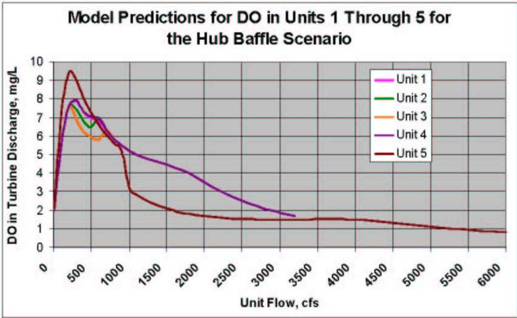
Figure 5: Predicted DO at Various Flow Levels for Each Unit Assuming Hub Baffles Have Been Installed on Units 1-5
