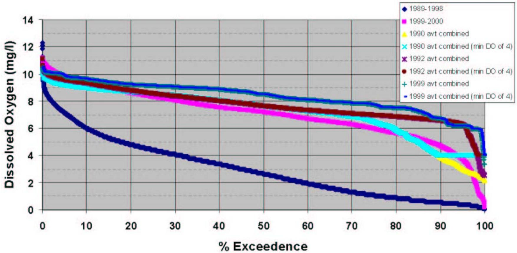
Figure 20: Percent of Time That Various Dissolved Oxygen Concentrations Would be Exceeded in Saluda Hydro Tailwater – for the Low DO Period (~7/1 – 11/15)
