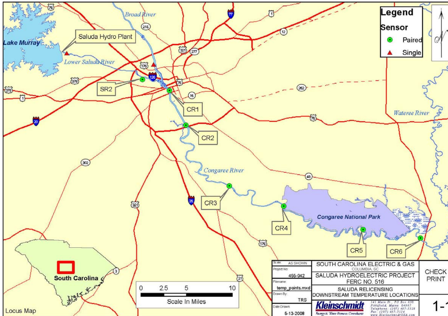
Figure 1-1: Map of Lower Saluda and Congaree Rivers Showing Location of Saluda Hydro Project and Temperature Sensor Deployment Sites
