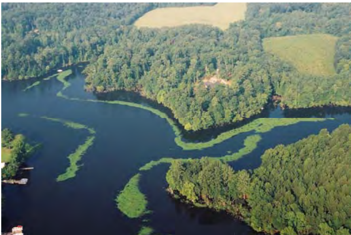
Figure 3. Water Primrose reaching the surface of the lake in 2005. The roots were at elevation 346 and had started growing during the drawdown of 2003-2004. When the pool increased over the winter of 2004-2005, the weeds were not killed during freezing conditions because they were submerged.
